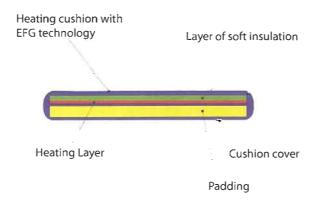
When a weight is applied to the cushion, the soft insulation layer is compressed, and heating energy begins to warm the person sitting on it.
